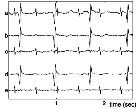
FIG. 20. Short segment from the original ECG (a), of the mother and fetus contributions estimated without delay embedding (b,c), and of the two contributions estimated with delay embedding (d,e).
